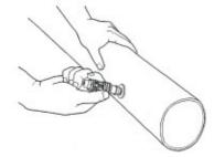
Insert and locate fitting firmly against flange of grommet and pull back slightly to seat the barb.
