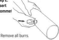
Place "TOP HAT" grommet firmly into hole with flange facing out.
