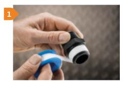
Apply PTFE tape or approved sealant to the male thread. Sufficient tape needs to be applied to ensure a watertight seal.
