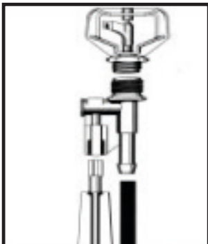
Threaded Stake Head and Combi Spike 5mm barbed bottom entry. Code HD5. Use with 5mm flexible riser tube connection to the lateral.
