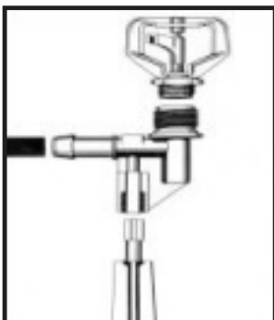
Threaded Stake Head and Combi Spike 5mm barbed side entry. Code HD10 & HD13. Use with 10mm or 13mm poly tube connection to the lateral.
