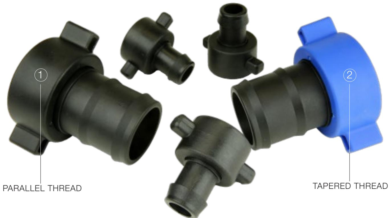
**(1) Parallel Thread (Black Nut)** – Also known as a fixing thread, this method relies on two parallel threads providing a strong connection plus a washer to achieve the seal. This version was originally designed to primarily fit metal threads. Because a seal is used there is no requirement for thread tape which means a quick and reliable connection.
