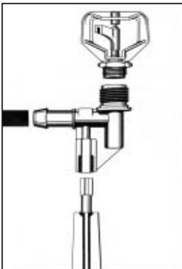
Threaded Stake Head and Combi Spike 10mm & 13mm Barbed side entry. Code HD10 & HD13. Use with 10mm or 13mm poly tube connection to the lateral.
