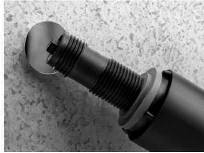
2. Remove the back nut from the bottom of the valve and insert the threaded section of the valve into the base of the cistern or small tank. Ensure the stem sleeve is in direct contact with the base of the tank so that it seals and prevents water from leaking.
