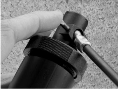
1. Insert the cam end of the lever assembly into the valve plunger recess. This may require rotation of the plunger to align it to the correct position. Align the cam hole with the valve housing and insert the pivot pin then flare the ends to secure.
